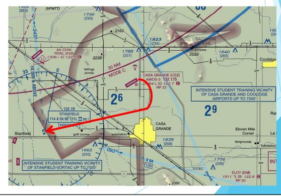
Due to risk of opposite direction approaches and frequent near mid air collisions, AFTW recommends that VFR training aircraft do not fly the GPS Rwy 23 approach into KCGZ.
